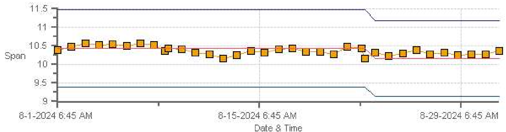
CH4[ppm] Calibration: PRAMP RENO-B Monthly: 08-2024 Type: SpanAndZero - Span
