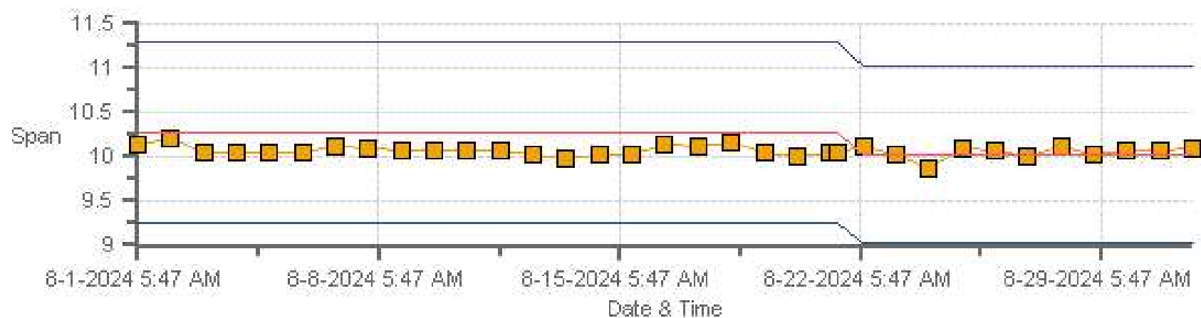
CH4[ppm] Calibration: AQHI Grimshaw Monthly: 08-2024 Type: SpanAndZero - Span
